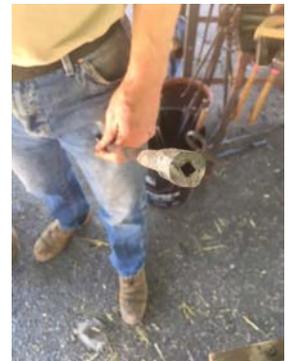
Martin Pansch forged a square hole that started out as a round hole, which he had drilled into the end of this bar. No drift needed. That was quite a nifty trick in moving metal.
